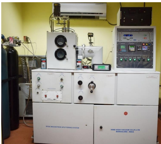
Fig. 3.4. The photograph of the sputtering system in our lab, used for synthesis of the nc-SiGe thin films.
