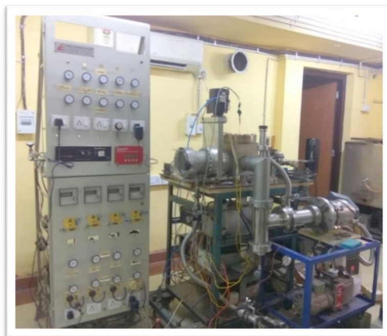
Fig 3.7. Real photograph of the 13.56 MHz CC-PECVD system.
