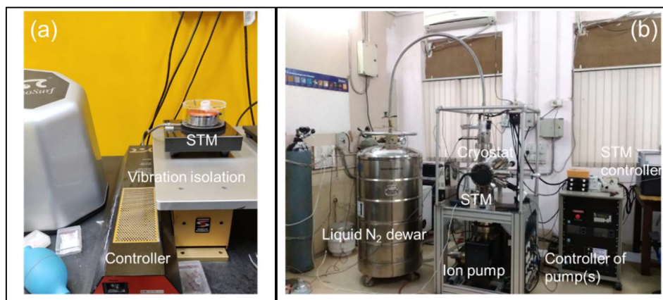
Figure 2.14. Digital image of (a) ambient (left panel) and (b) UHV STM (right panels) instruments used during this doctoral research.
