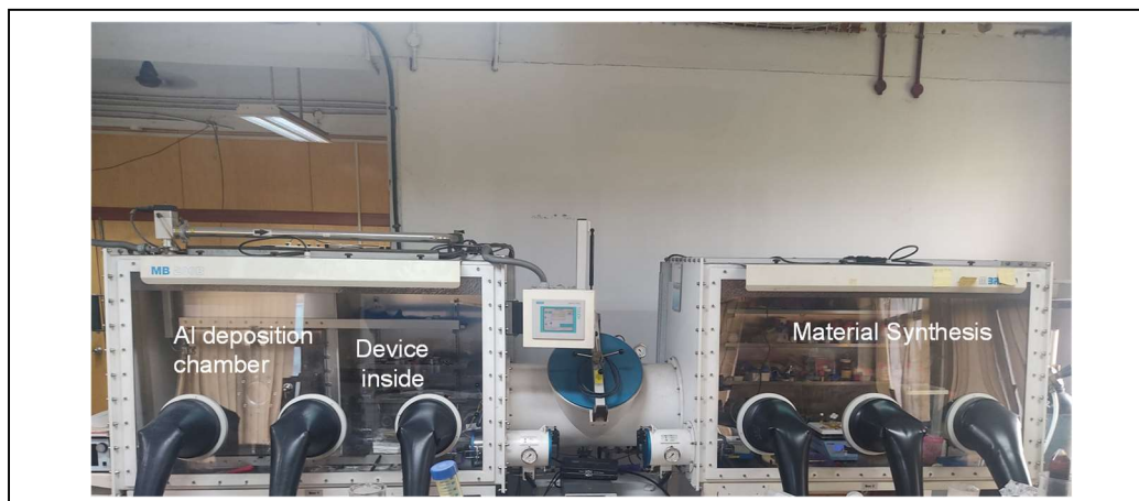
Figure 2.18. Practical set-up of solar cell measurements inside the glove box.
