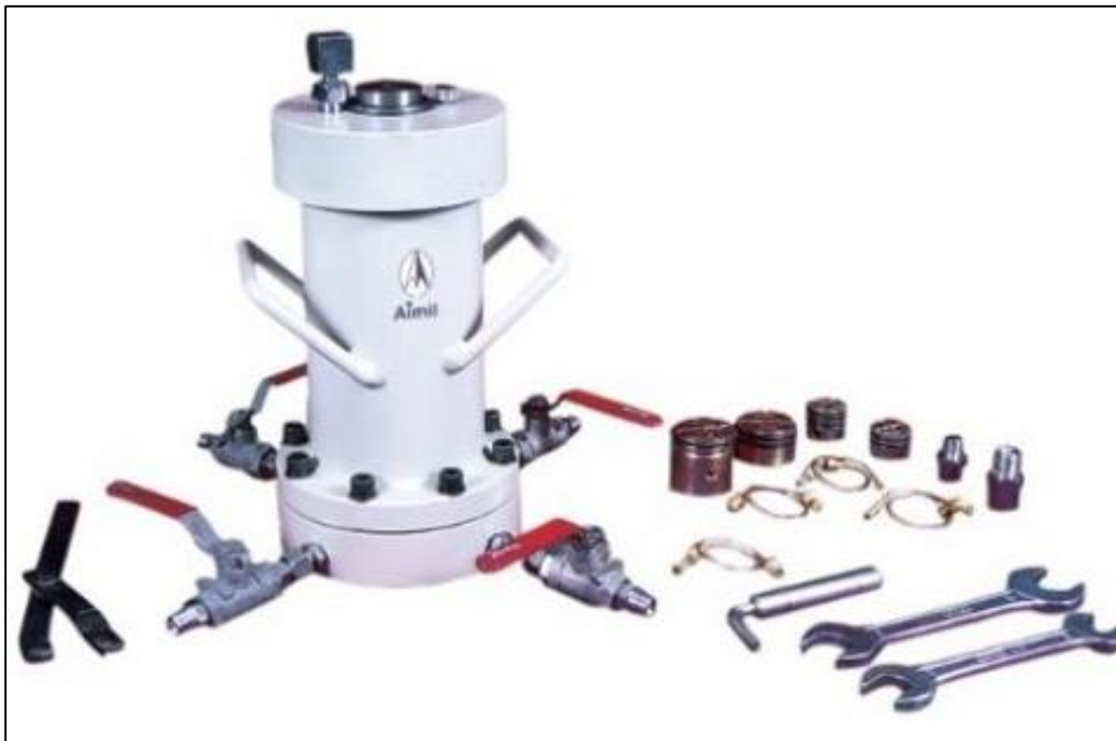
Figure 3.9. Sample assembly in Triaxial Test Outfit for Hard Material Testing
