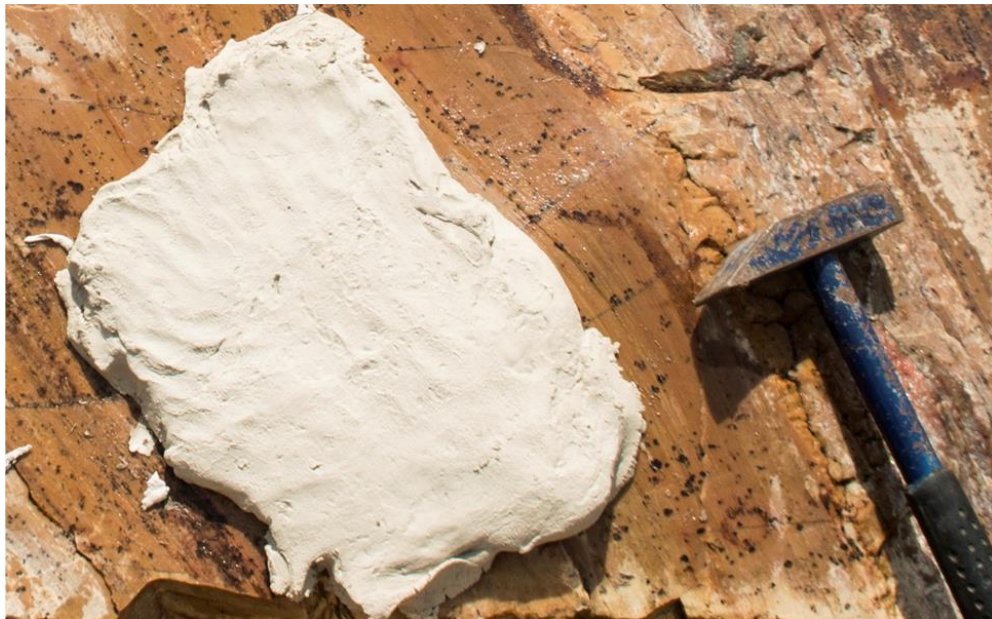
Figure 4.5. A plan view of the Plaster of Paris layer used to cast a natural fracture surface in quartzite.
