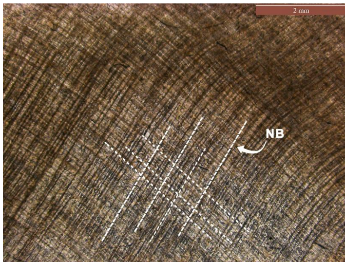
Figure 6.5. Uniform development of closely spaced, conjugate narrow bands (NBs) in homogenous PS models deformed at low strain rate ( \dot{\epsilon} = 2 \times 10^{-5} \text{ sec}^{-1} ). Note that strain rate doesn't have any effect on shear band formation in homogeneous model.
