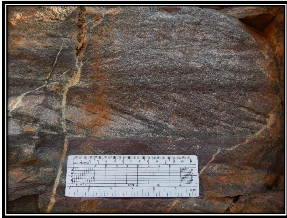
Fig 3.16 Ripple laminated sandstone facies from Kanampalli ( 14^{\circ}25'13.44'' N, 78^{\circ}05'25.06'' E) section, Gulcheru Formation, Cuddapah Basin, India representing solitary set of climbing ripple
