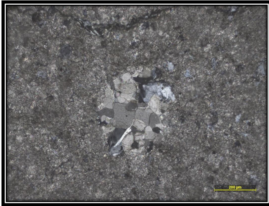
Fig. 5.7 KU-4 sample: Thick layer of shale with clustering of quartz grains in the middle
