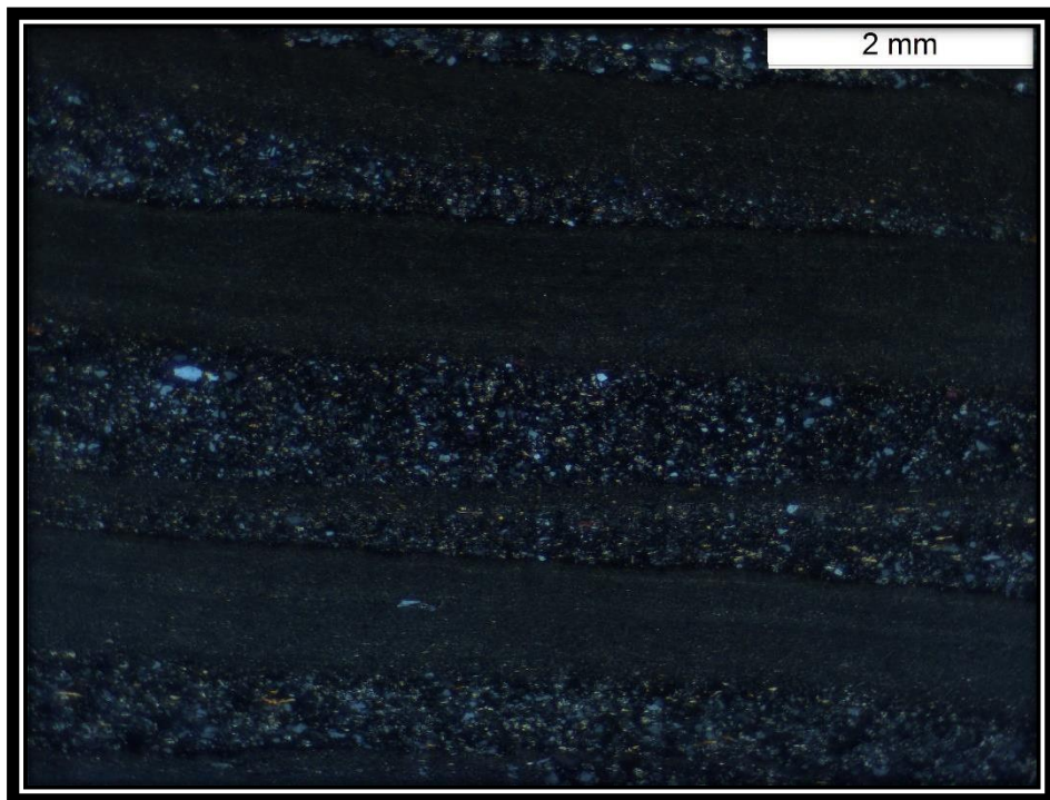
Fig. 3.35 Microscopic view of rhythmite facies showing graded clay layers with some lenticular silt layer
