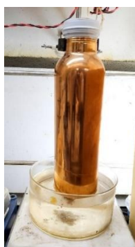
Figure 13. Experimental set up for reaction in copper bottle.
