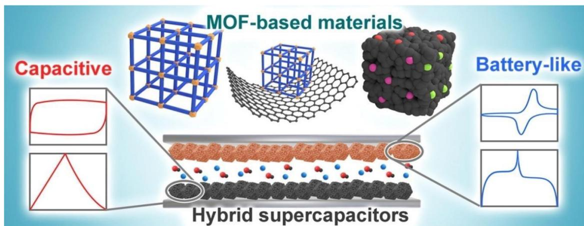
**Figure 1.16** Hybrid supercapacitor application of MOF-based materials.<sup>96</sup> Reprinted with permission.
