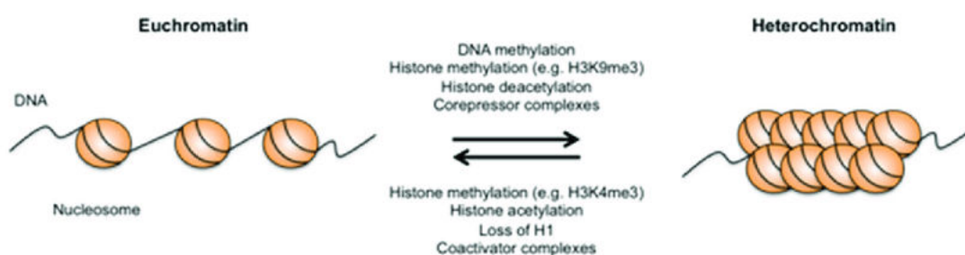
Fig. 26 : Schematic illustrating conformational transition between euchromatin and heterochromatin regulated by different epigenetic mechanisms. Euchromatin is open and accessible for gene transcription machinery whereas closed heterochromatin prevents transcription. Adapted from MOJ Cell Sci Rep. 2016;3(1):26–28.
