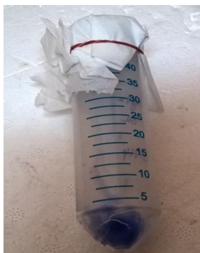
Figure 4.2 Bright blue cell pellets obtained after dye removal from the medium, indicating the adsorption of RBBR on the bacterial biomass
