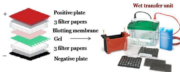
Fig.3.10. Arrangement of filter paper, gel, and membrane for western blot. (A) Semi-dry transfer (B) Wet transfer
