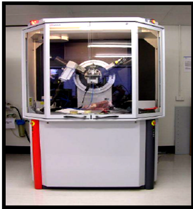
Fig. 3.4. X-ray powder diffractometer BRUKER D-8 ADVANCE (Department of Physics, Jadavpur University).
