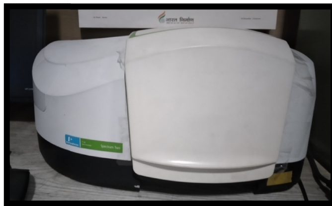
Fig. 3.8. FTIR spectrometer, Model : Perkin Elmer FT-IR Spectrum 2 spectrometer (Variable Energy Cyclotron Centre, VECC).
