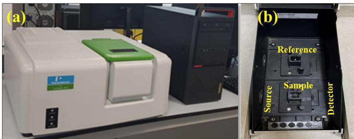
**Figure 1.14:** UV-Vis spectrophotometer instrument of the Dept. of Physics, JU; (b) sample chamber
