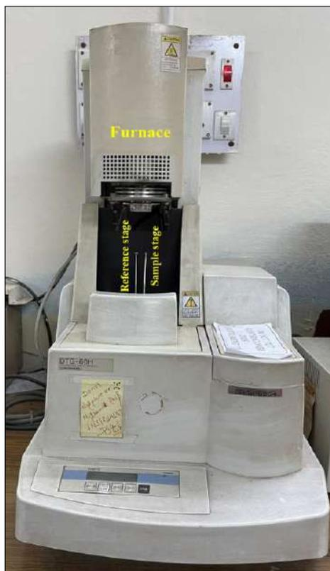
**Figure 1.13:** The DTA-TGA instrument of Dept. of Physics, JU
