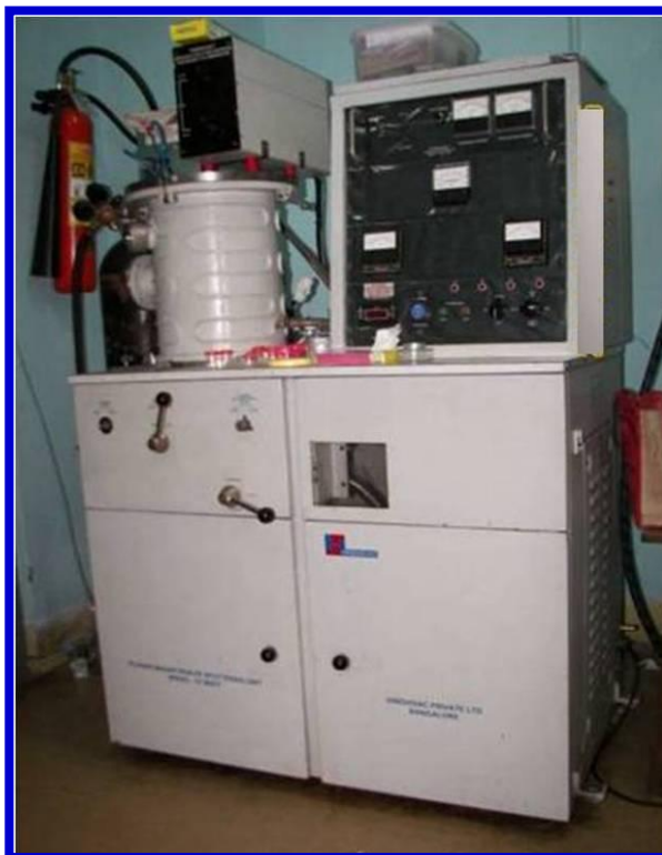
Fig. 3.4. Photograph of the RF-magnetron sputtering unit used here (HindHivac, Bangalore, India (Model: 12" MSPT))
