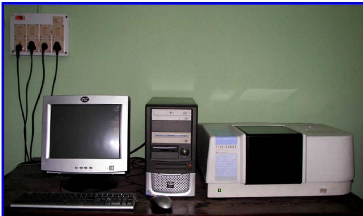
Fig. 3.16. Digital image of the FTIR spectrometer (Here, Shimadzu FTIR-8400S spectrometers were used for IR spectroscopic analysis)
