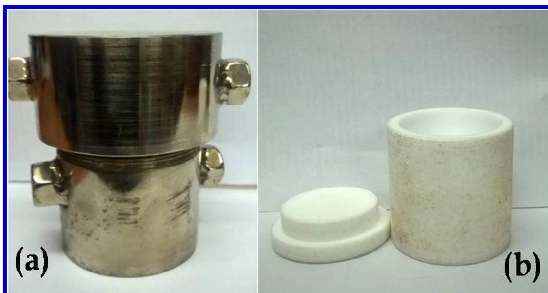
Fig. 3.1. (a) Autoclave arrangement and (b) Teflon tube inside the autoclave used here
