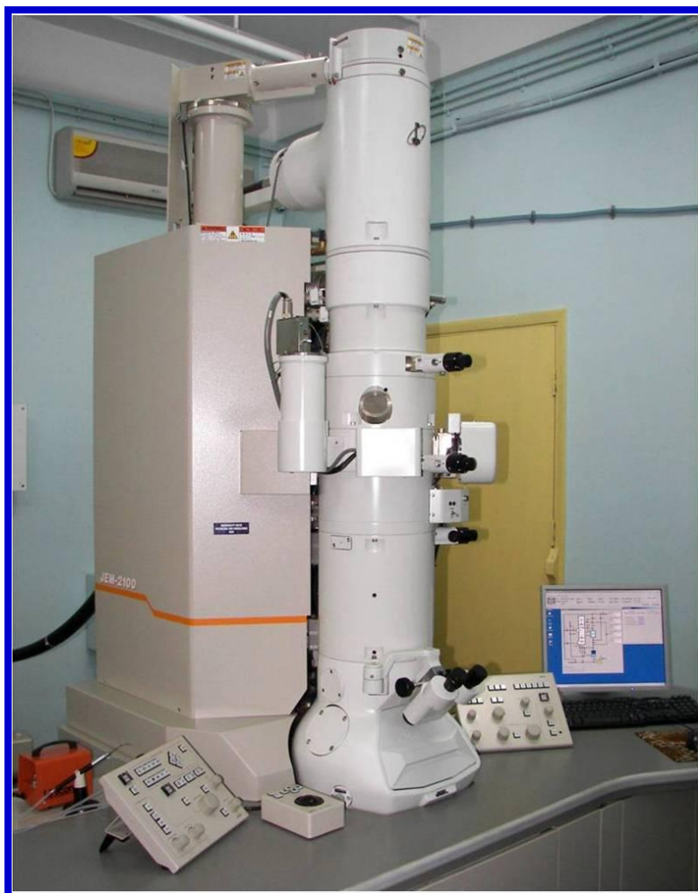
Fig. 3.8. Digital photograph of HRTEM instrument having phosphor screen and sample holders in left and right insets
