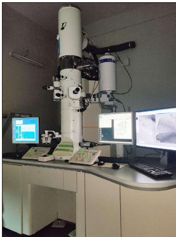
Figure 2.5 The HR-TEM facility of IACS, Kolkata used to obtain the TEM micrographs
