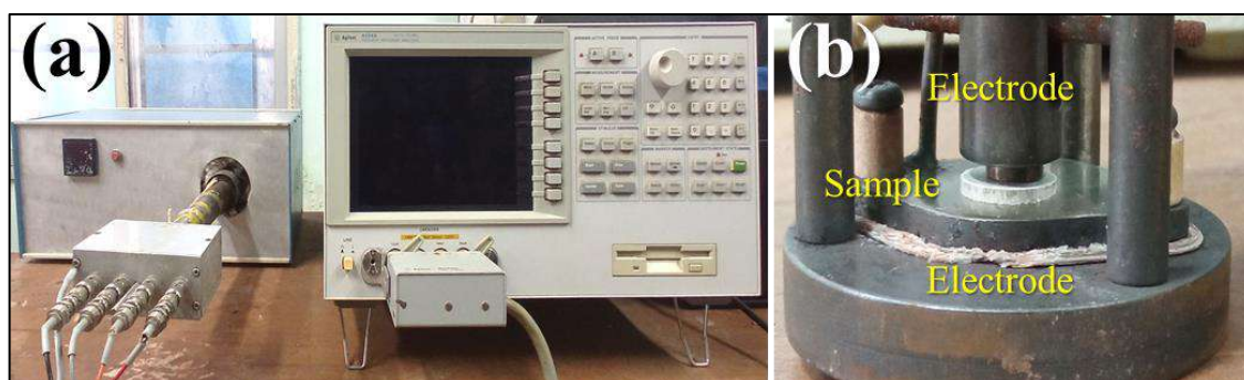
Figure 2.10 (a) The Agilent impedance analyzer set up of the Dept. of Physics, JU, (b) the electrode system with the contacts of the instrument
