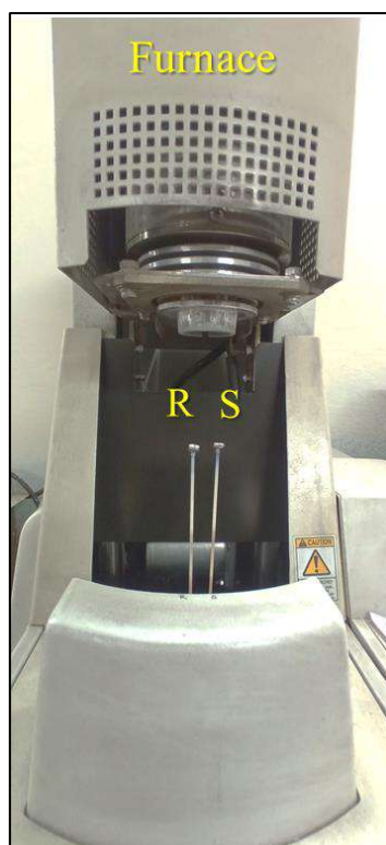
Figure 2.7 The DTA-TGA instrument of Dept. of Physics, JU showing the furnace, reference (R) and the sample (S) stages.
