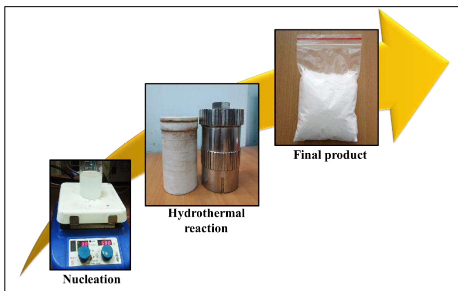
Figure 2.1 General synthesis procedure of boehmite nanoparticles
