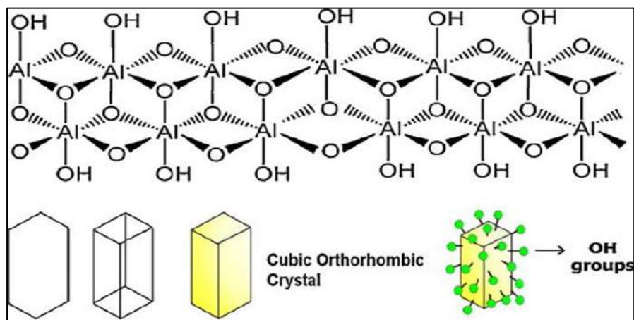
Figure 1.10 The orthorhombic structure of boehmite (Source: Vatanpour et al., J. Membrane Sci. , 401, 2012 pp.132-143)
