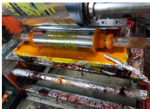
Fig 6.3: Engraved Gravure Cylinder during printing on blister foil
