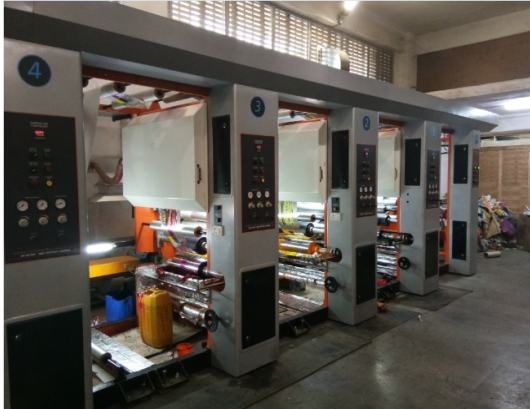
Fig4.4: 4-Colors(CMYK) gravure printing machine
