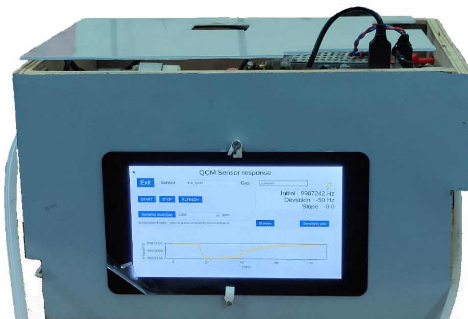
Fig. 3.7. The developed portable gas sensing system.
