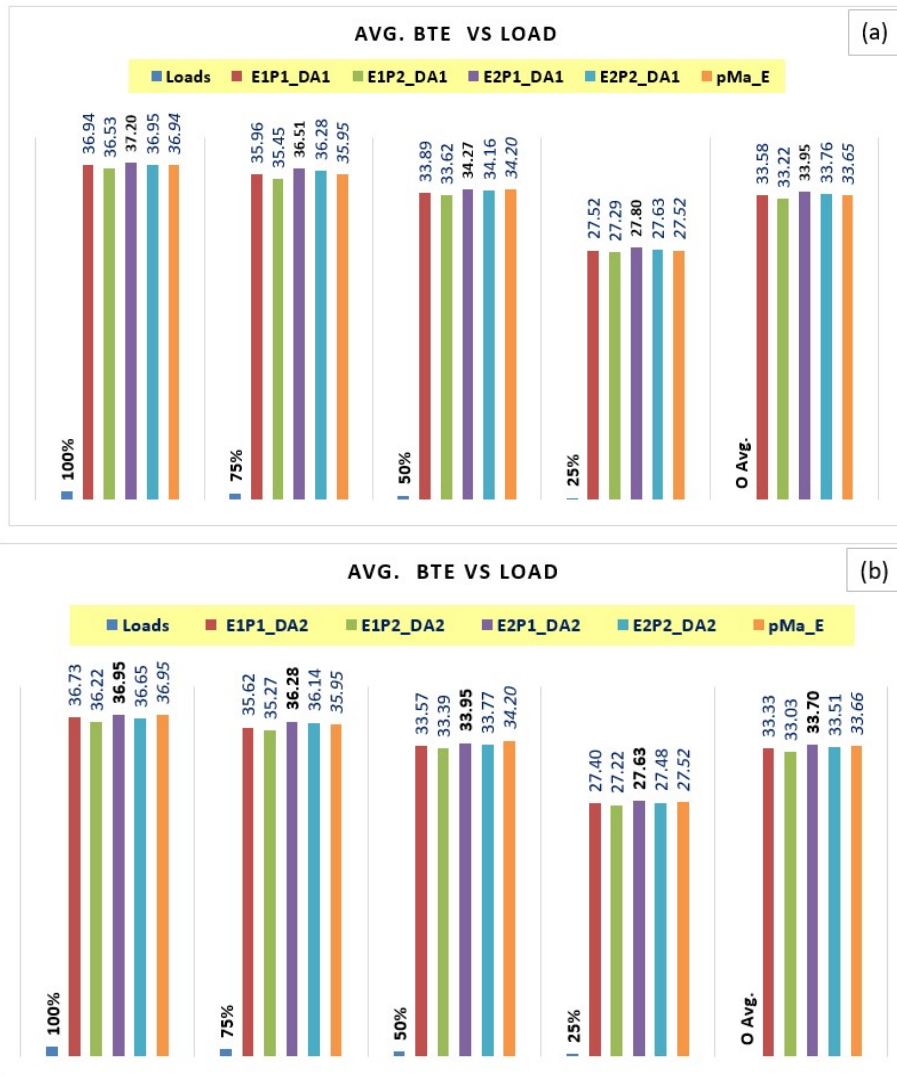
Figure 8.10:- Average BTE data with variation of Load and post injection dwell (a) 1100 ms & (b) 1300 ms
