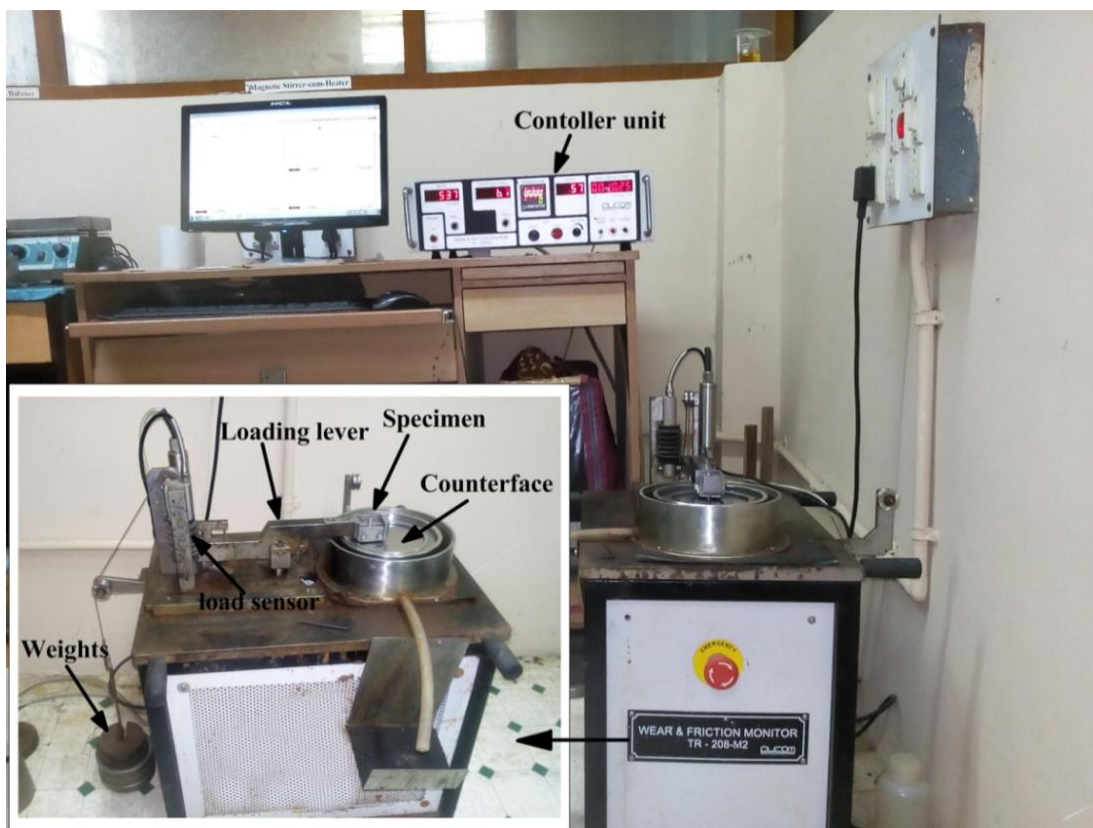
Figure 2.7: Pin-on-disk tribotester (TR-208-M2, DUCOM)
