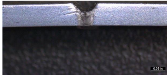
Figure 6.5 Undercut seen on the welded sample at a peak power of 4.75kW.
