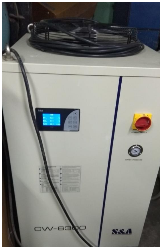
Figure 3.6 Chiller unit of laser welding machine
