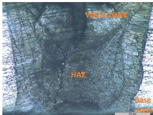
Figure 5.9 Image showing the weld zone along with heat affected zone and parent material at high power.
