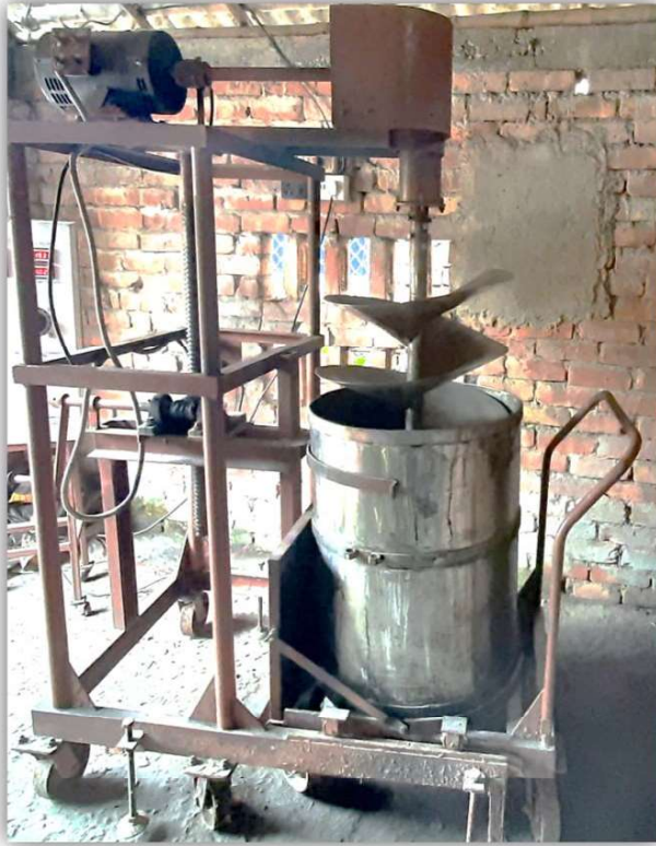
Figure 12: Operational view of the presented drying unit. Position of the mixing spindle is raised up before loading
