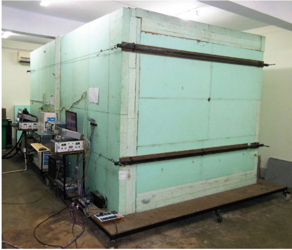
Fig. 2.2 Guarded Hot Box Test set-up installed at laboratory ( D. Chowdhury et. al 2019 ).
