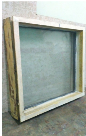
Fig. 3.24 DGU placed in wooden frame.
