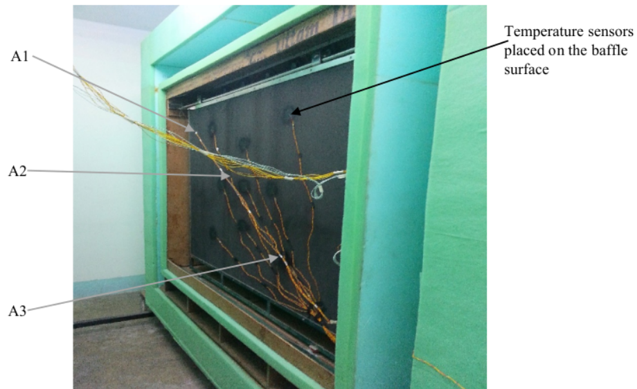
Fig. 2.10 Location of air temperature sensors (A1, A2 & A3) in the metering box
