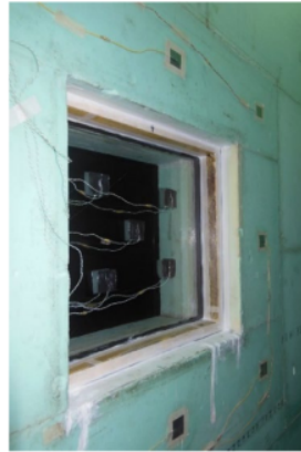
Fig. 3.26 Sample WV placed in the surround panel with thermocouple sensors mounted.
