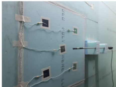
Fig. 2.16 Hot wire anemometer setup for measuring air velocity
