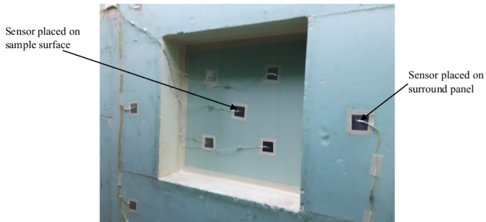
Fig. 2.11 Temperature sensors placed on the surround panel and sample surface ( D.
