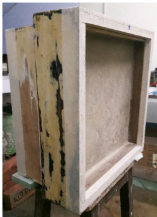
Fig. 3.4 Sample WI – 125mm brick wall with 12.5mm plaster inside sample holding frame
