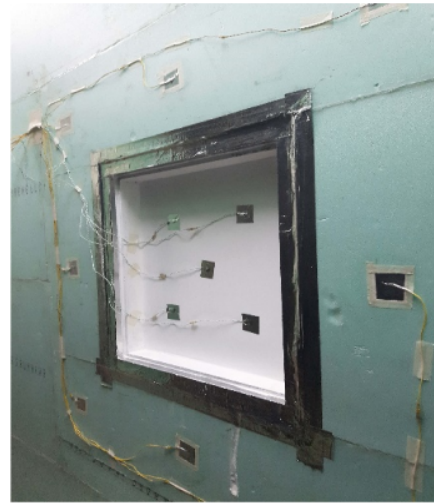
(b) Sample WII mounted on surround panels
