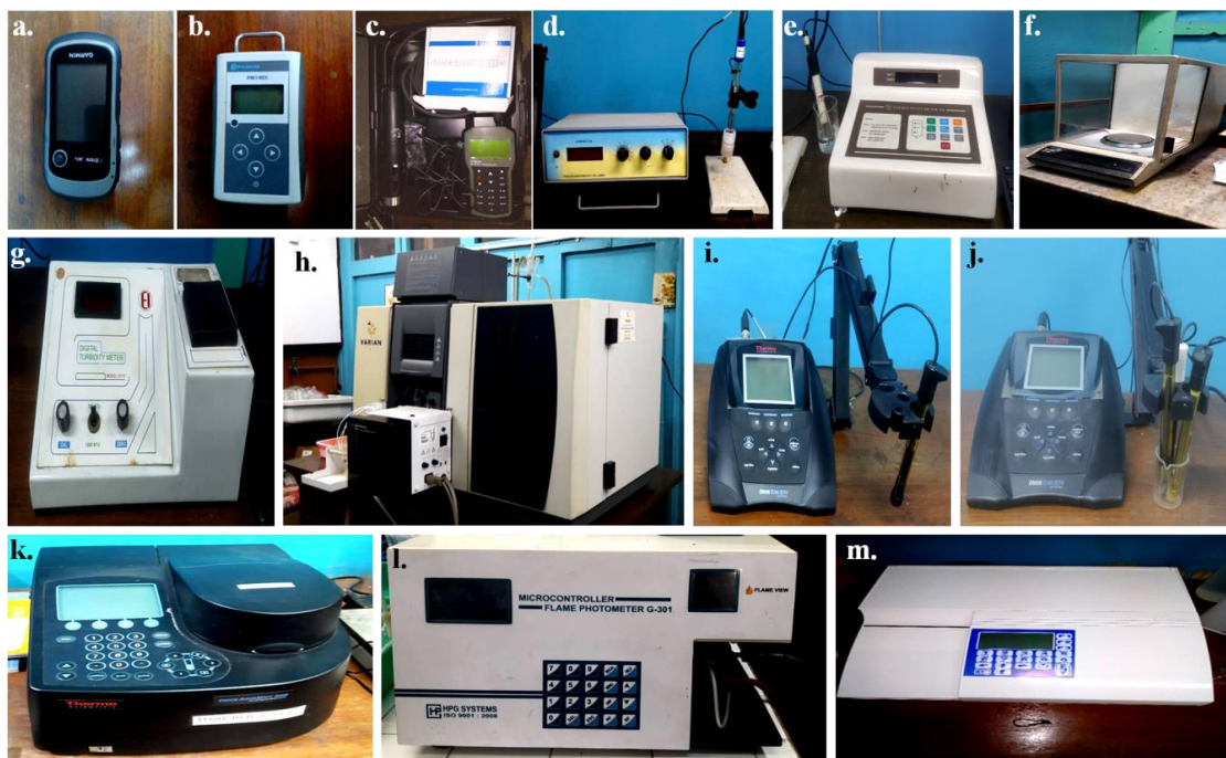
Fig. 12. Instruments used to analyze different physico-chemical parameters: (a) GPS meter, (b) Radiation meter, (c) HANNA multiparameter, (d) pH meter, (e) Conductivity meter, (f) Fine balance, (g) Turbidity meter, (h) Atomic Absorption Spectrophotometer, (i) Ion selective electrode for Fluoride, (j) Ion selective electrode for Nitrate, (k) UV-Vis Spectrophotometer, (l) Flame photometer, (m) Fluorescence spectrophotometer
