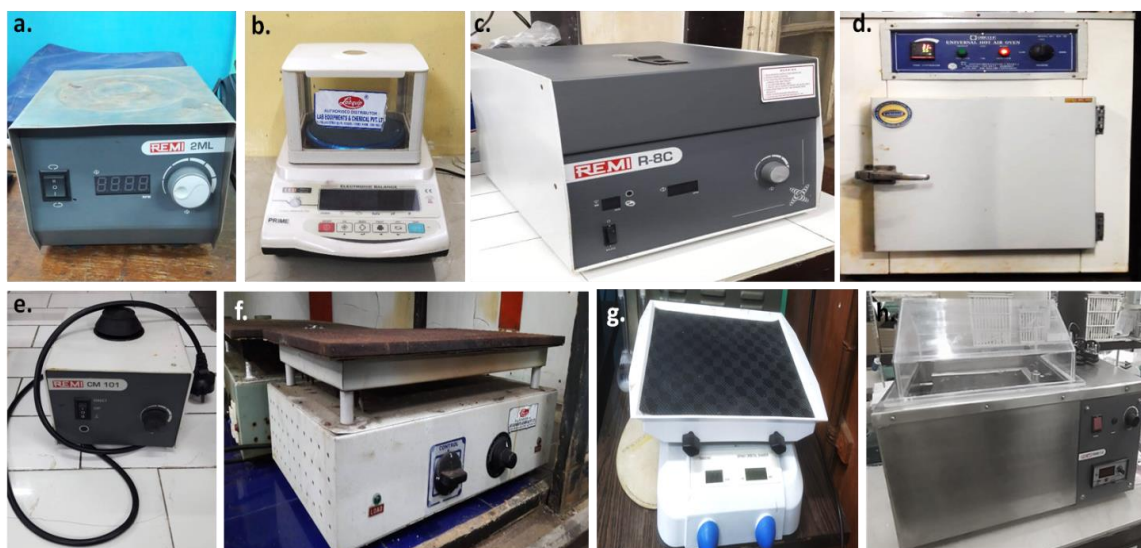
Fig. 13. Instruments used during sample processing: (a) Rough balance, (b) Magnetic stirrer, (c) Centrifuge, (d) Hot air oven, (e) Vortex, (f) Hot plate, (g) Orbital shaker, (h) Water bath
