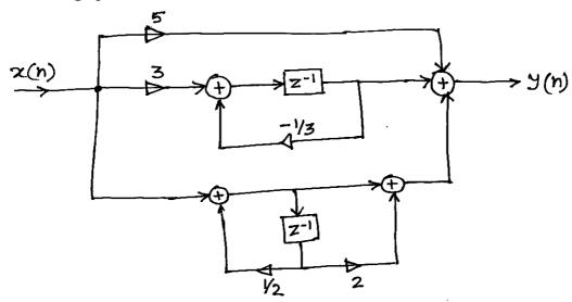
(b) Compute the impulse response and the step response of a DT LTI system described by the following difference equation.
