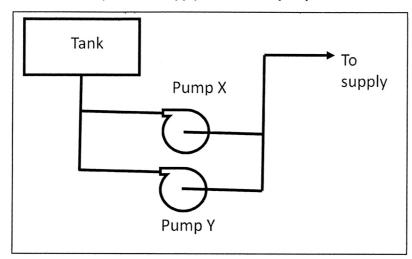
failure. The mechanical failure rate of pump X and Y are 0.25 yr<sup>-1</sup> and 0.1 respectively whereas the electric supply failure rates to the pumps is 0.1. Construct a fault tree and then estimate the failure rate to supply water. (10)
