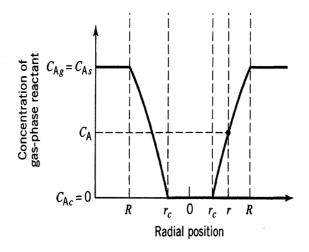
R= radius of the particle;  $r_c$  = radius of unreacted core
