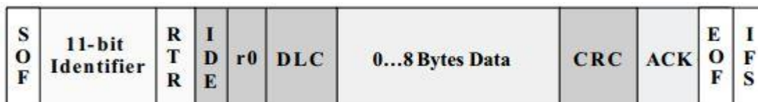
Figure. 3.5 (a): CAN Data Frame for Standard (11 bit identifier) Format
