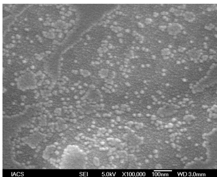
Figure 6.13a: Scanning electron micrograph of freshly prepared lyophilized liposomes L3.
