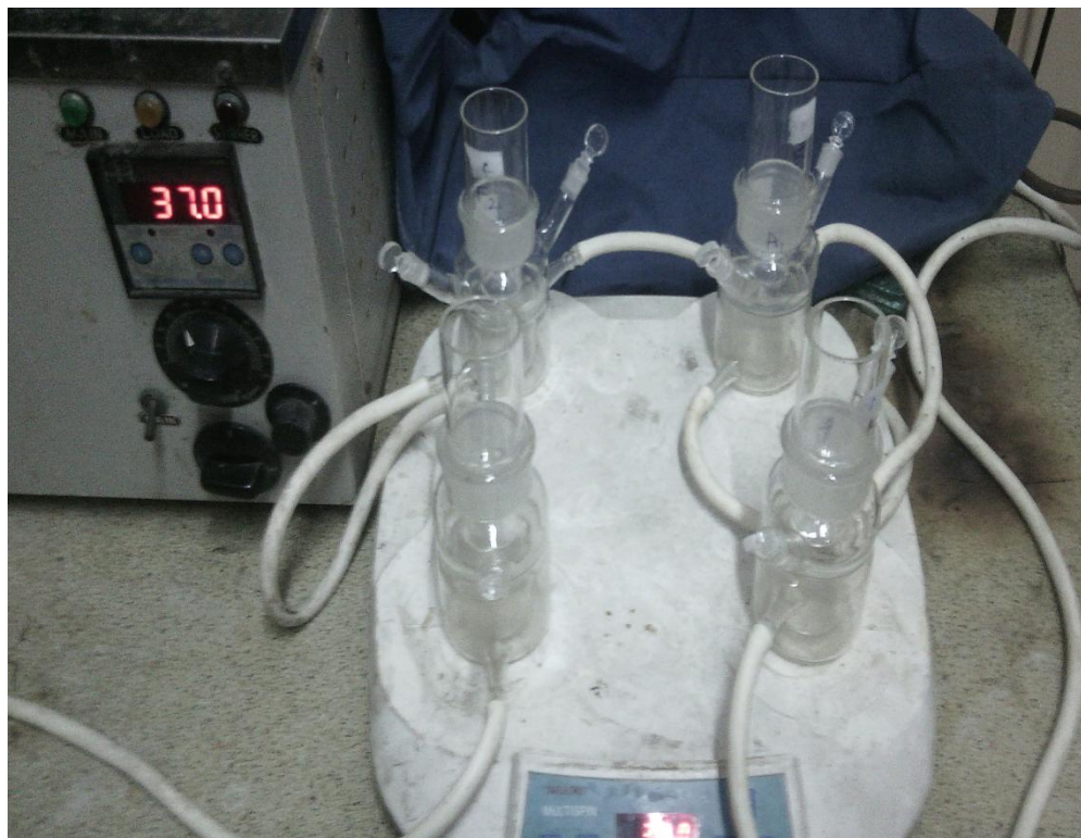
Diffusion and permeation study done in Franz diffusion cell in the Laboratory
