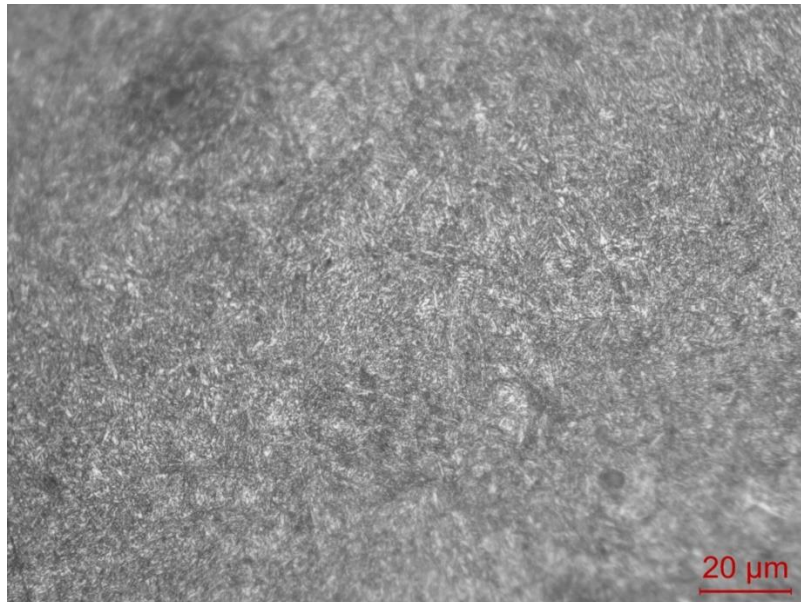
Fig. 4.3.3.b: [100 X Etchant-2% nital ] The microstructure taken at cross section shows pancake structure of ferritic and pearlitic grains.
