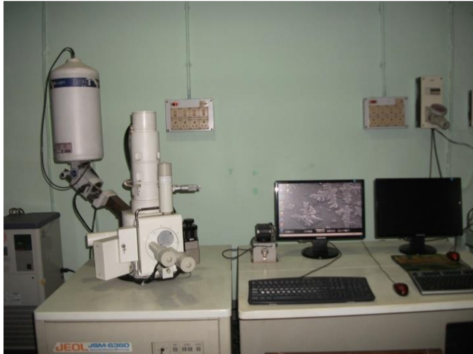
Fig 3.1.3 SEM used while performing the tests.
