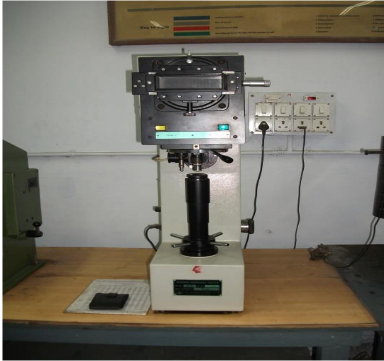
Fig 3.1.4 Macro-hardness tester used -VM 50
