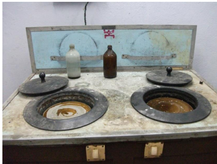
Fig.3.1.1.c Polishing of specimen in polishing wheel
