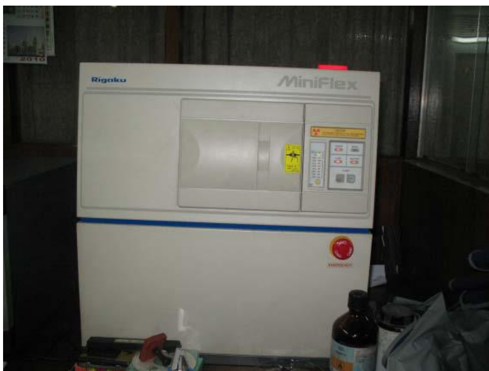
Figure 4.3: Rigaku X-ray diffractometer with Cu target (Miniflex, Japan)
