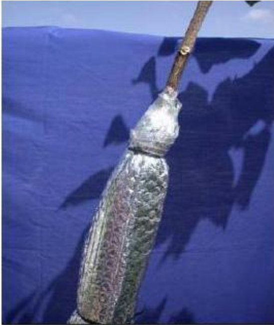
Step 9: secure shield below the sensor
