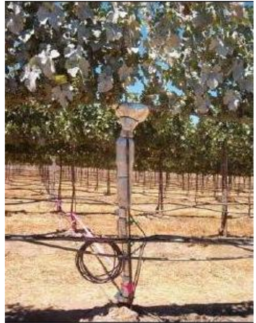
Step 10: Second wrap at cordon 'T' over all wrapping stem below sensor wrapped in thin foil or bubble shield
