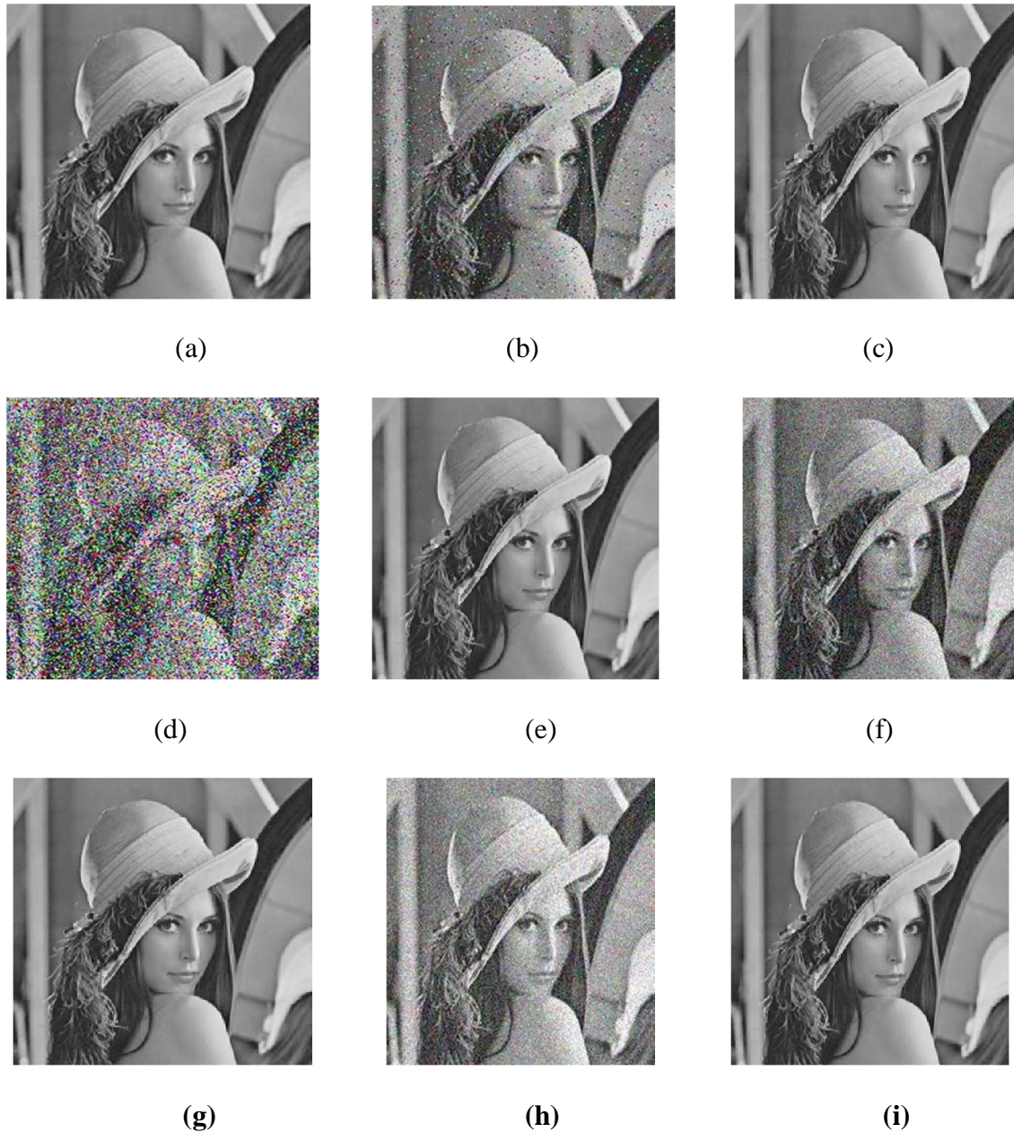
Figure 27 (a) A benchmark image of Lenna, (b) Image corrupted with 0.04 Salt & Pepper Noise, (c) Image restored after BFO, (d) corrupted with 0.4 Salt & Pepper Noise, (e) Image restored after BFO, (f) Image corrupted with Gaussian Noise at S.D.= 0.004, (g) Image restored after BFO, (h) Image corrupted with Gaussian Noise at S.D.=0.07, (i) Image restored after BFO.
