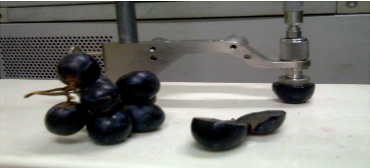
Fig. 4.8 Dielectric parameter measurement of black grape with Agilent 85070E Dielectric Probe Kit and VNA
