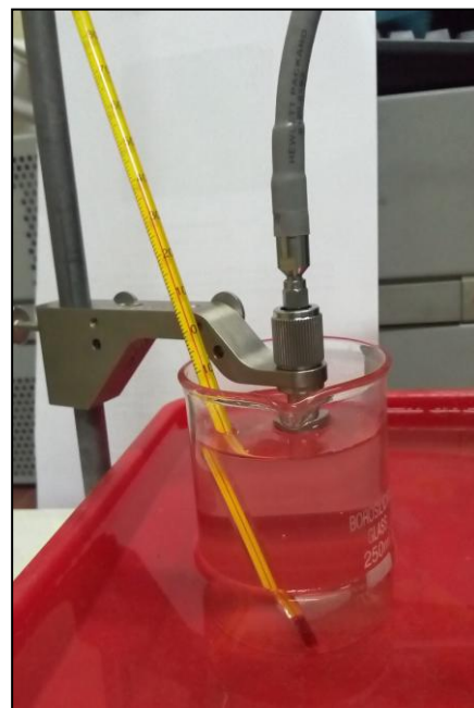
Fig.6.1 Measuring temperature of the phantom liquid using thermometer when the beaker is placed in hot water
