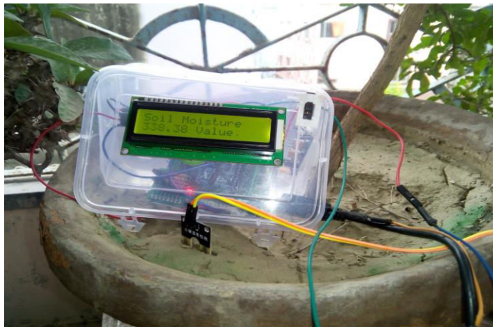
Fig. 3.27 Experiment Set-up with Soil Moisture Sensor in dry soil and its output on LCD
