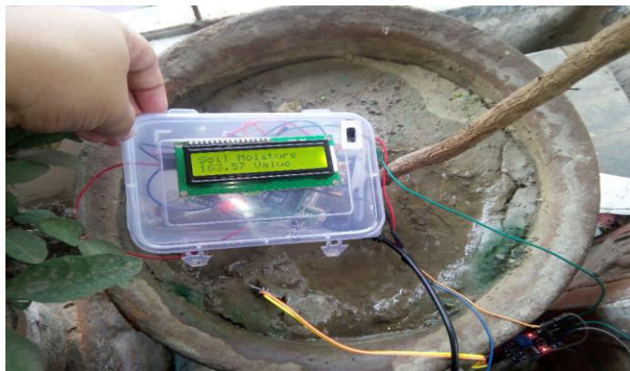
Fig. 3.28: Experiment Set-up with Soil Moisture Sensor in wet soil and its output on LCD
