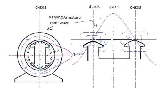
$$\begin{split} X_d > X'_d > X''_d; \quad X_q = X'_q; \quad X'_q \gg X''_q \ and \ X''_d < X''_q \\ X_d = x_a + X_{md}; \quad X'_d = x_a + \frac{1}{\frac{1}{X_f} + \frac{1}{X_{md}}}; \quad X''_d = x_a + \frac{1}{\frac{1}{X_f} + \frac{1}{X_{md}} + \frac{1}{X_{kd}}} \\ X_q = x_a + X_{mq} = X'_q; \quad X''_q = x_a + \frac{1}{\frac{1}{X_{mq}} + \frac{1}{X_{kq}}} \end{split}$$
