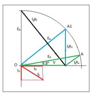
$$E_o = V_{ph} + j I_1 \times (0.8 - 0.6j) \times X_s$$
