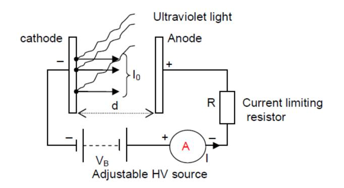
Consider a simple electrode arrangement as shown in the Fig., having two parallel plate electrodes (representing uniform field geometry) separated by a distance d and immersed in a gas at pressure *p*. A uniform electric field *E* is applied between two electrodes. Due to any external radiation (ultra violet illumination) free electrons are liberated at the cathode.
