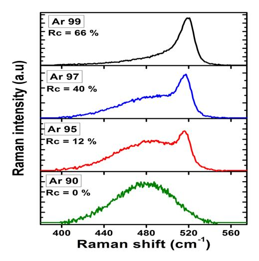
> As we increase Argon dilution, crystalline fraction increases and material changes from amorphous to nanocrystalline to microcrystalline phase.
