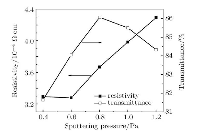
**Variation of Resistivity and Transmittance with Power for ITO**
