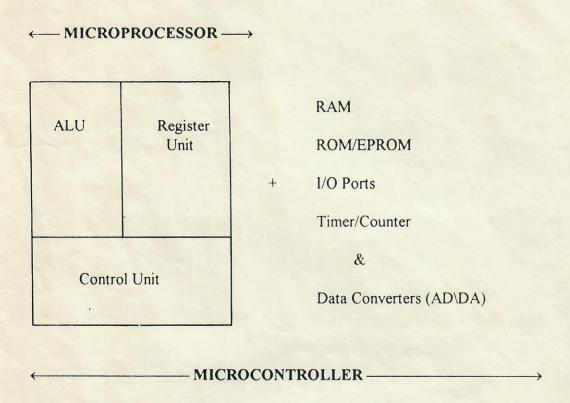
Fig. 1: Block diagram of Microcontroller
