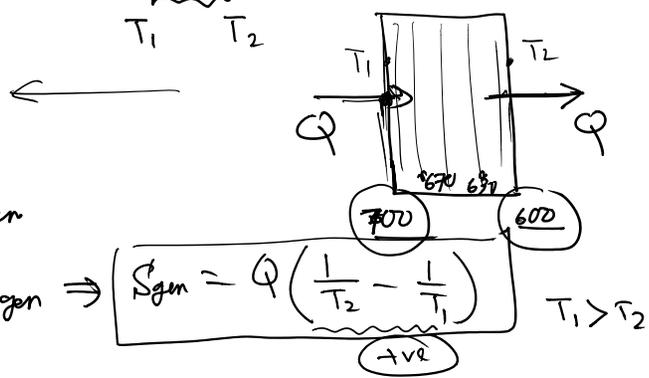
$0 = Q \left( \frac{1}{T_1} - \frac{1}{T_2} \right) + S_{gen} \Rightarrow S_{gen} = Q \left( \frac{1}{T_2} - \frac{1}{T_1} \right)$
