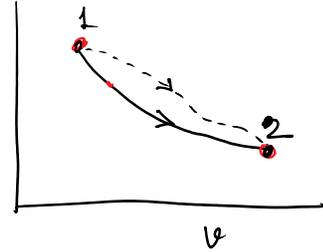
$$\int_1^2 \left( \frac{\delta Q}{T_b} \right)_{rev} = S_2 - S_1$$
