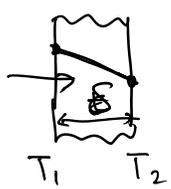
$\dot{Q} = kA \left( \frac{T_1 - T_2}{\delta} \right)$
