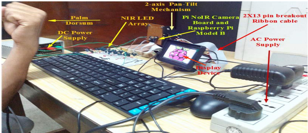
Figure 4.1. Complete Integrated System Developed for Real-Time Human Recognition Using PDSVP [80]
