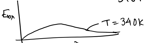
Blackbody Emission Spectrum from the absorber plate
