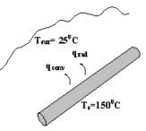
Problem 4: Find the radiation heat transfer coefficient for a polished aluminium whose temperature exceeds that of surrounding( $T_{sur}=25^{\circ}C$ ) by  $10^{\circ}C$ . Emissivity value for the surface may be taken as 0.05.
