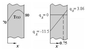
T=T<sub>max</sub> where  $\frac{dT}{dx} = 0$  and  $\frac{d^2T}{dx^2}$  is negative. This happens at *x*=0.75 m
