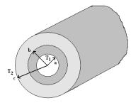
Problem 7: A cylinder with heat generation given by q has been exposed to surroundings at 25 °C. The convective heat transfer coefficient outside is h=15 W/m<sup>2</sup>K. Outer surface emissivity is 0.8. Find q so that the temperature of outer surface is kept within 200 °C. Also find temperature distribution inside the cylinder and T (r = 0). Given that k = 25W/mK,  $r_0 = 25$  mm
