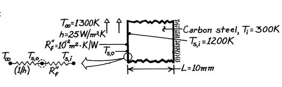
Heating of coated furnace wall during start-up.
