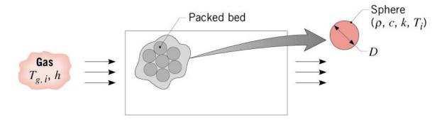
**KNOWN:** Diameter, density, specific heat and thermal conductivity of aluminum spheres used in packed bed thermal energy storage system. Convection coefficient and inlet gas temperature.
