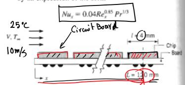
Estimate the surface temperature of the chip if it is dissipating 30 mW.
