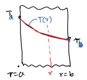
$$T_0 = C_1 \ln a + C_2$$
