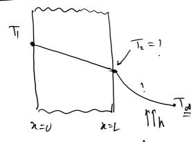
$$T(x) = T_1 - \frac{hx}{k+hL} (T_1 - T_{\omega})$$
