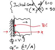
B) Zero Heat flux  $-k\frac{\partial T}{\partial n}\Big|_{n=k_{1}} = 0$   $\frac{\partial T}{\partial n}\Big|_{n=k_{1}} = 0$   $\frac{\partial T}{\partial n}\Big|_{n=k_{1}} = 0$   $\frac{\partial T}{\partial n}\Big|_{n=k_{1}} = 0$ prevails
