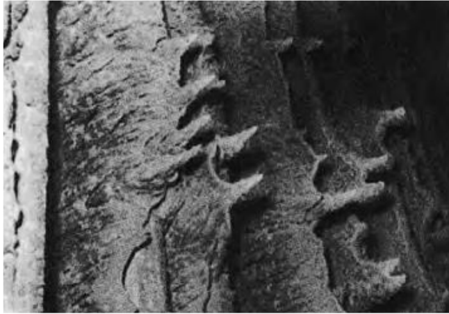
Fouling of ash on SH tubes
