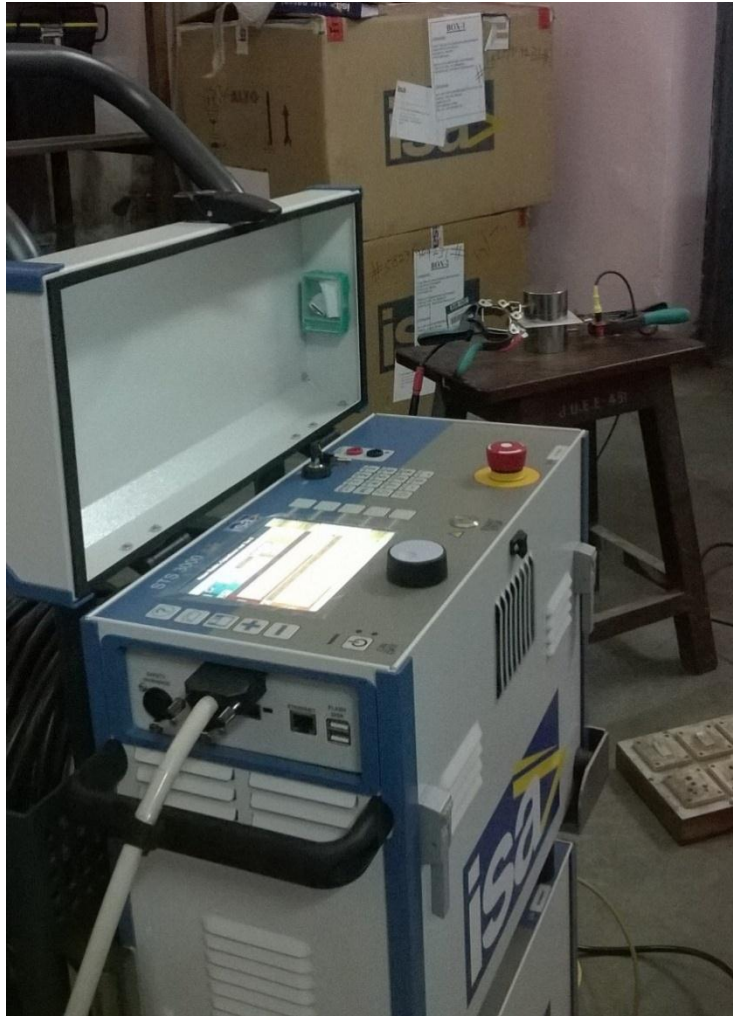
Figure 4.11.measurement setup for tan delta & capacitance in High Voltage Lab
