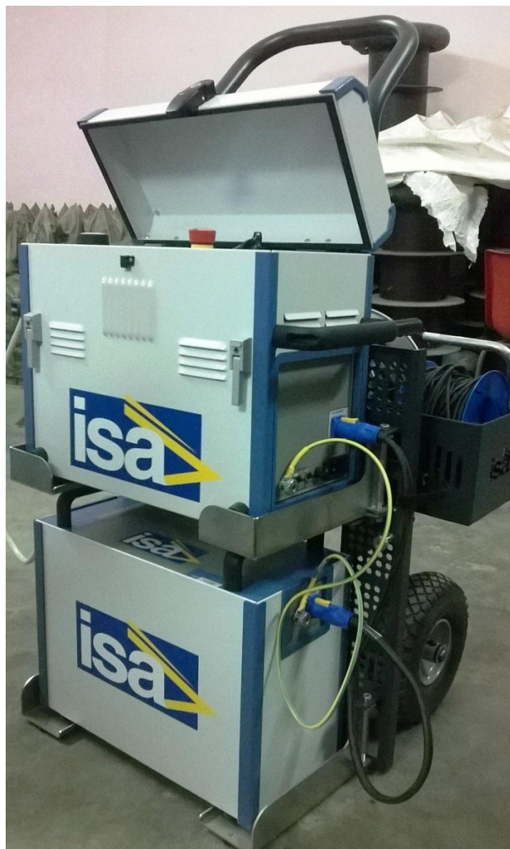
Figure 4.9 TDS 5000 tan delta and capacitance measurement device
