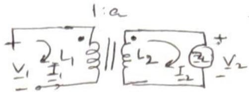
sinusoidal s.s.  $\underline{V}_1 = \underline{I}_1 j\omega L_1 - \underline{I}_2 j\omega M$
