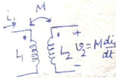
Dot convention: Current entering dotted terminal of one coil produces ~~an~~ an open ckt. voltage
