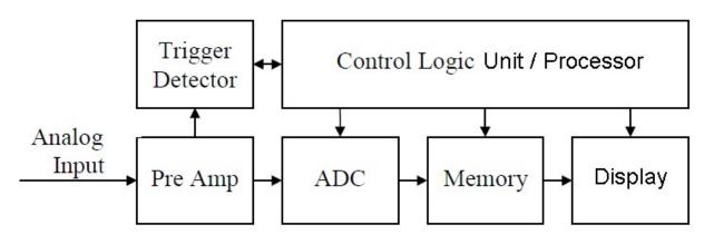
A Digital Storage Oscilloscope (DSO) uses digital memory to store a waveform. In order to do this the incoming signal must first be digitized, once this is complete the data in the memory can be continuously replayed through a digital to analogue converter and displayed on a CRT. Unlike analogue storage scopes the captured waveform does not decay over time.
