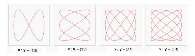
(Frequency of X input) : (Frequency of Y input) = (No. of tangents to y axis) : (No. of tangents to x axis)
