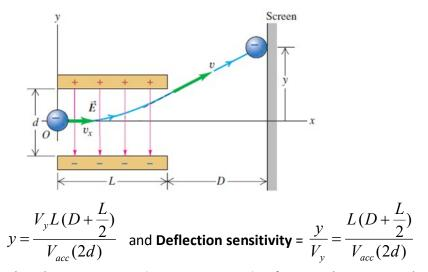
3. <u>Time base generator (sweep generator</u>): If we apply a sawtooth signal  $V_x(t) = kt$  to the horizontal input, the horizontal screen axis will be proportional to time t. In this case a signal  $V_y(t)$  applied to the vertical input, will depict on the oscilloscope screen the time variation of the signal.
